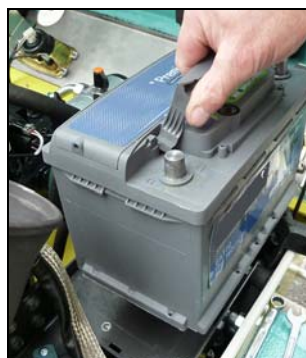
Fig. 10-2 Replacing the battery
