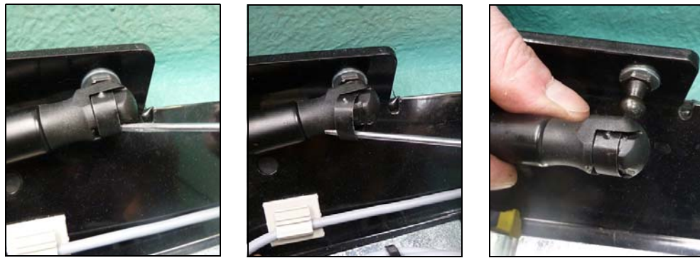
Fig. 10-5 Using a screwdriver, lift the clips and loosen the springs
